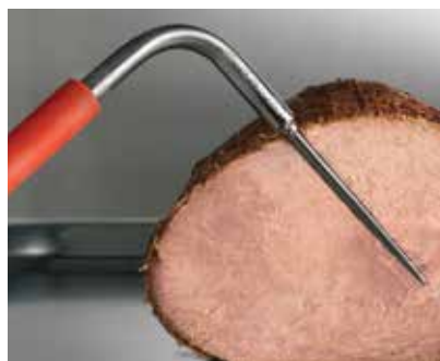
Multi-sensor food probe with 3 sensors.
